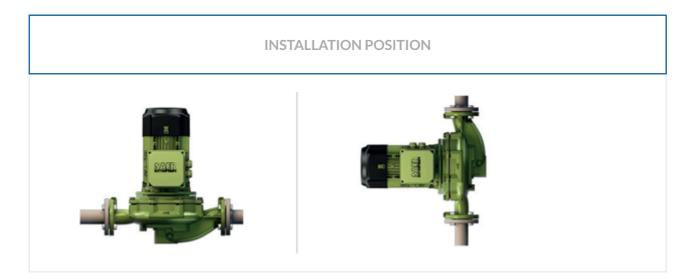
Both installation positions are possible (always with the motor upwards)
